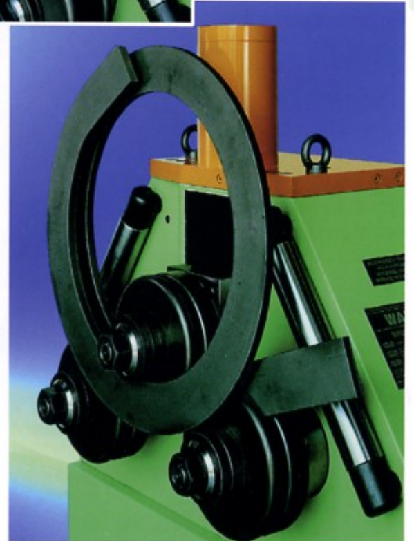
Standard rolls bending flat bar hard way
