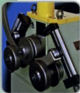
Leg-in Angle Rolling Tools Available on All Models
