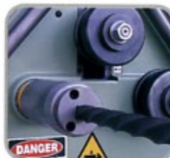
STANDARD Twist Tool w/Collet and Clamp
